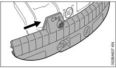
Slide the lower guide slot of the skirt onto the deflector – it must snap into position.
