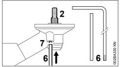
The output shaft (2) must be blocked with the stop pin (6) or screwdriver (6) to mount or remove cutting attachments. These parts come standard with the machine or are available as special accessories.
