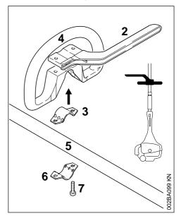
► Place the clamp (3) in the loop handle (4) and position them both against the drive tube (5).
