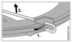
► Disconnect wire rod from the transport guard.
