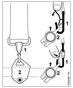
Press down the bar on the carabiner (1) and pull the carrying ring (2) out of the carabiner.
