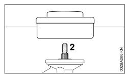
Only mowing heads may be used which mount directly to the shaft (2).
